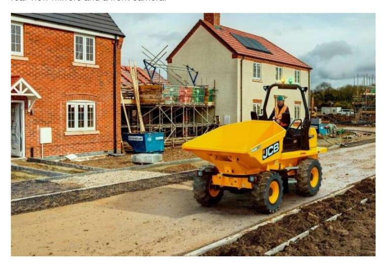
JCB's new 6T SiteSafe ROPS dumper has a maximum machine weight of 4,500kg and therefore meets the EN474 revisions with a rollover bar.
