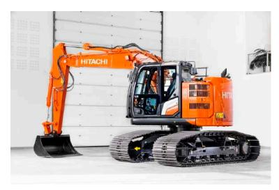
With compact dimensions and added protection, it is designed for applications such as logging and log felling as well as digging and loading. It is assembled at the Hitachi Construction Machinery (Europe) factory in Amsterdam.
