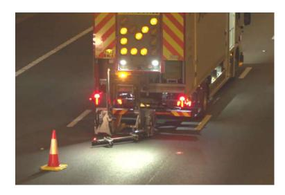
The Falcon ACLM automated cone laying machine is being deployed by Balfour Beatty's Connect Plus Services' consortium, which looks after the M25 for National Highways.
