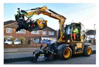
Coventry City Council has invested in a JCB PotholePro following a trial last summer when it repaired more than 100 sqm of road in just two hours – an area the council says would normally take four days to fix using traditional methods.
