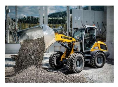
redesigned operator's cab, with more glass than ever – right down to the foot well – to give an unobstructed view of lift arms and attachments.
