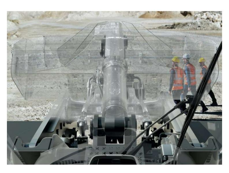
Owing to blind spots caused by the buckets on wheel loaders, the area in front of the machines has been considered an area of major concern in terms of safety. With the new Doosan transparent bucket function, however, the driver can easily check the blind spots in front of the bucket via the cab monitor, to increase safety and prevent accidents.
