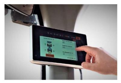
Tyre monitoring has also been improved. The new tyre pressure monitoring system (TPMS) has individual sensors that mount to the valve stem of each tyre along with a receiver module that communicates the pressure for each tyre onto the display and alerts the operator when the tyre pressure is outside of a set range.
