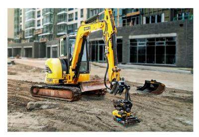
Tiltrotator manufacturer Engcon has developed a quick hitch system for attachments on excavators as small as two tonnes.
