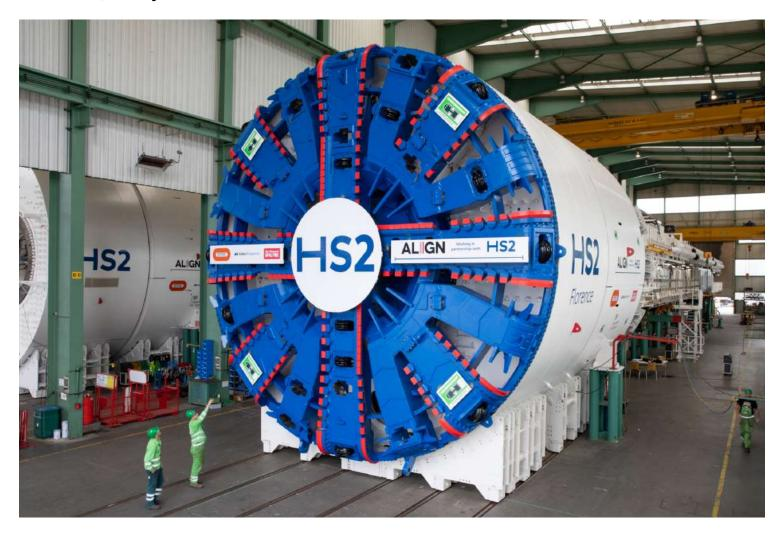
The TBMs have been made by Herrenknecht in southwest Germany. At 2,000 tonnes and 170 metres long, they were transported to the UK in more than 300 separate shipments over the course of two months.
